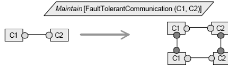
Fig. 6. Fault-tolerant refinement pattern
